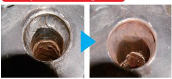
Removing scale adhered to inside of a heat exchanger in a pressure molding machine (three months after)
