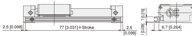
The "With sensor rail" model is shipped with the sensor rail and sensor magnet assembled on the piping port side.
