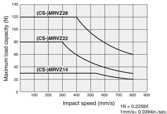
In the graphs, "Impact speed" refers to the speed immediately before the slider impacts the rubber bumper or shock absorber. This is not the same as "average speed (cylinder stroke/travel time)".
