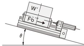
Note 2: When descending, heavier loads can be carried using lower operating air pressure (P) than when ascending.
