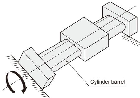
6. When mounting the body, always secure it by mounting bolts at 4 counterbore holes on the end plate (left and right).
